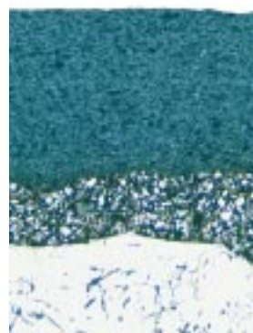
Cross section of Flygt epoxy coating
