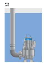
A semi-permanent free standing installation. Transportable version with pipe or hose connection.
