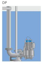
For semi-permanent wet well installations. The pump is installed with twin guide bars on a discharge connection.
