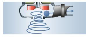
The powerful pumping action of the vortex impeller enables easy passage of liquids and solids.
