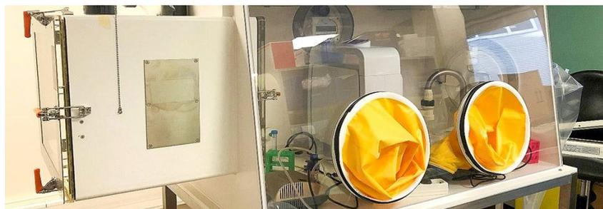
This 99.6% efficiency was achieved via a standard EOLIS Air Manager 600S equipped with a Perform+ filter unit including a **HEPA 13 filter** certified according to **NF EN ISO 29463-4 (formerly NF EN 1822-4)**. An aerosol of droplets contaminated with a known concentration of coronavirus was nebulised for five minutes in a hermetically sealed enclosure. The 99.6% abatement rate was then measured after only ten minutes of air treatment at the low speed 2 setting.
