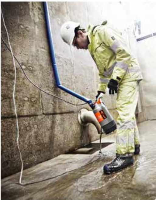
Minimised back flush: A special Ready 4L feature is the built in non-return valve to prevent so called back-flush. The water is kept inside when the pump is turned off or lifted up. When the pump is started, a valve disc opens up and lets the water pass through until the water is gone, or until you turn off the pump. When the valve disc closes, it goes down and seal against the lip-ring on low suction base and prevent water to flush out.
